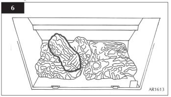
5.5 There are two ash panels which lay across the front of the burner skin. Place the panel with the flat edge facing the left side of the firebox. There are location holes on this log which fit over the screw holes of the burner skin.
